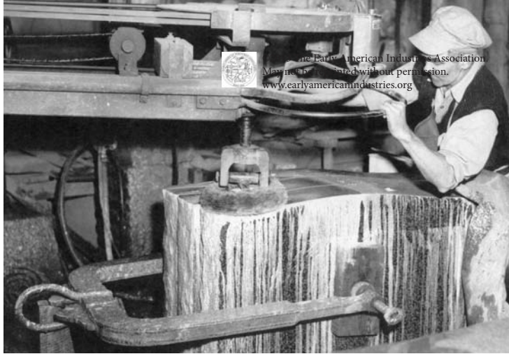
Figure 30 (above, left). Polisher with counterbalancing electric motor (to the left and out of the photo). The granite worker is using a buffer to simultaneously polish the serpentine tops of three dies that are clamped together.
