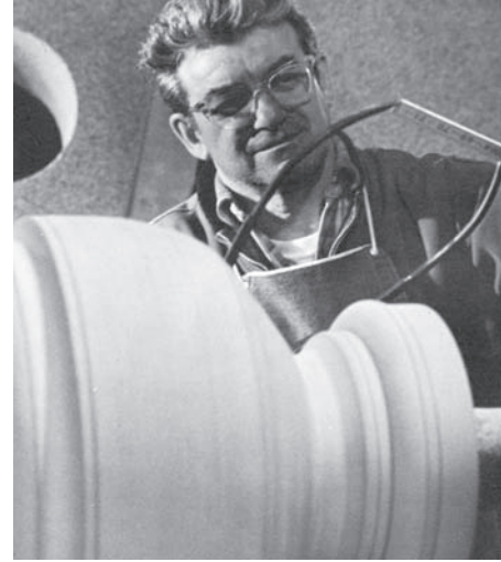
Figure 3 (left). Polishing lathe at the Woodbury Granite Co. Note the cast iron grinding blocks on top of the rotating column and extra blocks stored in front.
