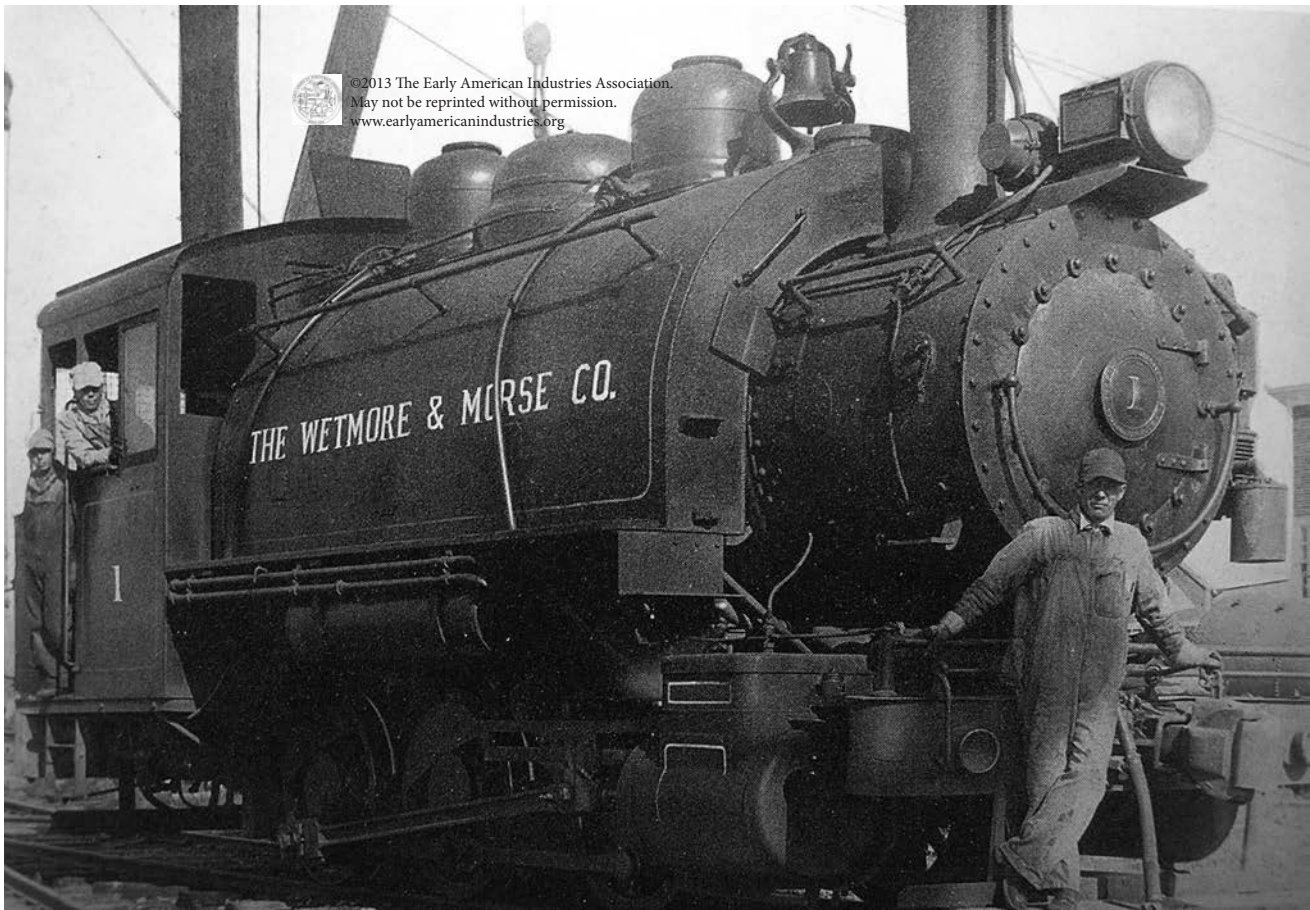
Figure 37 (above). Saddle tank locomotive at the Wetmore & Morse quarry at Barre, Vermont.
