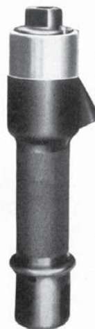
Figure 28 (above, left). The hand facer or “bumper” was a powerful hand-held pneumatic tool that could remove large amounts of granite in a short time. Its numbing effect on granite workers’ hands caused the granite workers’ union to lobby for its banishment.
