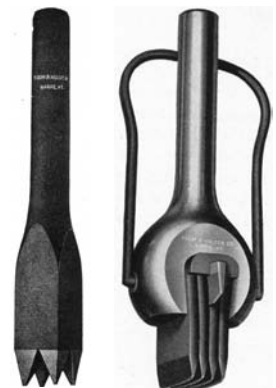
Figure 25 (far right). Pneumatic surfacer bush chisel used for the final stages of surfacing. Note the built-in operator handle.
