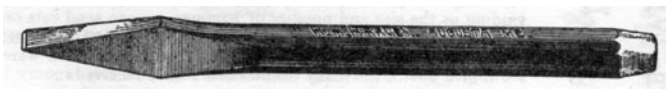
Figure 4. Cape chisel. The cape chisel is still used today by masons to remove old mortar in preparation for repointing.
