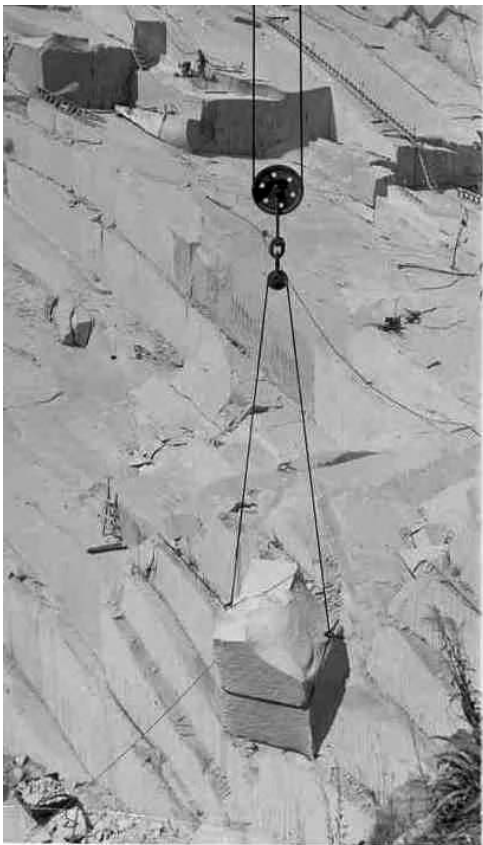
Figure 15 (above). A choke hitch.
