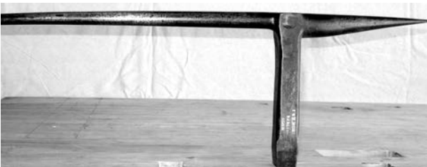
Figure 19 (above, left) A candlemold stake marked "J. & E. NORTH / BERLIN / CONN" circa 1824-1840, 24 inches long.
