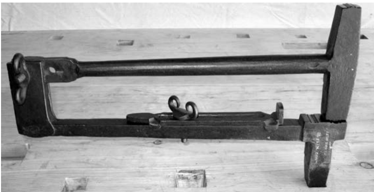
Figure 24 (right). A creasing swedge with two hammers made by Wilcox & Roys Sawpit N.Y., 1834.
