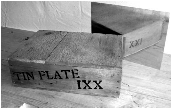
Figure 6 (above). A reproduction wooden box for shipping tinplate. This box holds 225 sheets of 10-by-14 inch tinplates. The IXX indicates the that base weight of the contents is 150 pounds.
