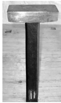
Figure 15 (left). A square stake marked "J. & E. NORTH / BERLIN CT" circa 1835-1854; 5 inches x 2½ inches at top.
