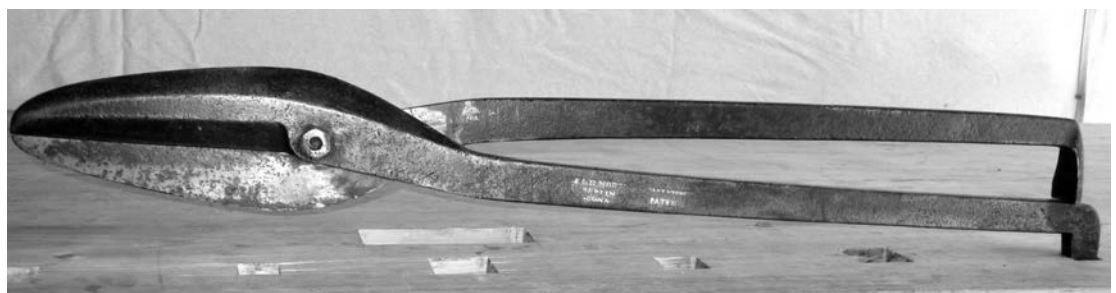
Figure 11 (right). A bench shear made by "J. & E. North Berlin Conn." circa 1824-1840, 29 inches long.
