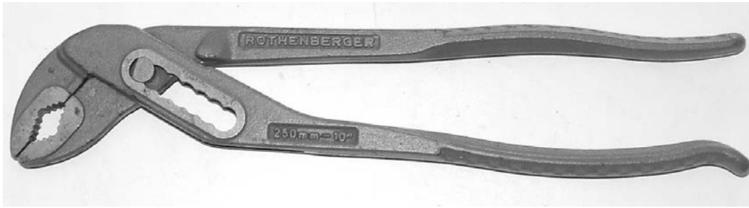
Figure 41 (left, top). A 10-inch Rothenberger model Nr.7.0528, boxed, slip-joint pliers with obtuse V jaws. Unlike the Footprint, this tool is entirely drop-forged.
