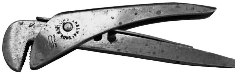
Figure 23. Ellin's patent improved Footprint. Apparently, this was the first production plier-wrench not requiring dismantling to change positions.
