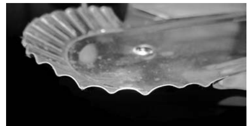
Figure 12 and detail (above). A scone formed using all three swedges (Figures 22-24). The curve on the top of the scone was formed with the creasing swedge. The fluted top edge was made with the square-pan swedge. The decorative triple bead that was added on the bottom and on the vertical edges was made using the cullender swedge. Wire was inserted along the vertical edges of the scone to strengthen it. The edges of the scone were turned on a hatchet stake and then the wiring stake was used to set the wire within the turned edges.
