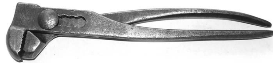
Figure 26 (below). J Schlehr's patent 10-inch, 90-degree parrot jaw, bolt holder. It is marked "Eagle Claw Wrench Co., Rockford, Ill. Pat'd Feb. 6. 1912" and has five sockets.
