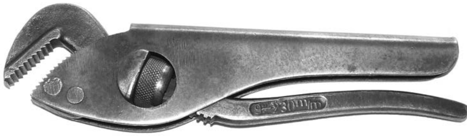
Figure 65 (left). A Henry Boker stamped, roll-nut offset footprint. The inner handle is embossed "9"—230m/m." It probably dates from the 1960s. The 1975 as well as current catalogs show 7-, 9-, and 12½-inch models.
