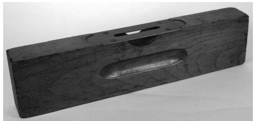
Figures 7 a and b (right). A Stanley no. 102 cherry level (two views) with original glass vial showing the Bodmer and Traut's patent on the level plate.
