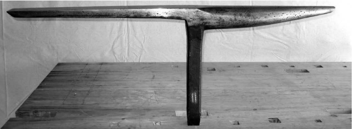
Figure 17 (above). A beakhorn stake marked "J. & E. NORTH /BERLIN CT" circa 1835-1854, 40 inches long.
