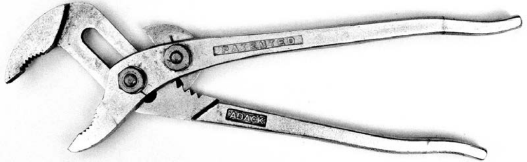
Figure 66 (below). A 9-inch chromium/vanadium steel "ADACK" "PATENTED" (no numbers) external rack-and-dog pliers. It is marked "MADE IN GERMANY."
