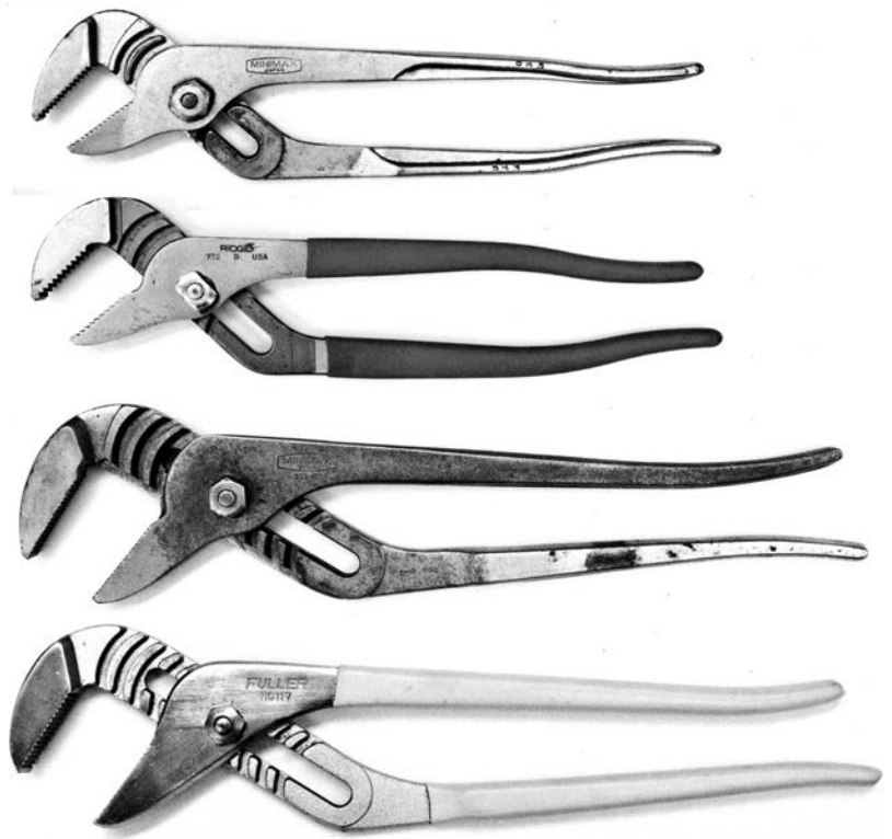
Figure 62 (right). Some heavyweight groove-joint pliers. A 12¼-inch Minimax 583 with seven settings, Japan; a 12½-inch Rigid 732 with seven settings, USA; a 16-inch Minimax 359 with ten settings, Japan; and a 16½-inch Fuller 117 with ten settings, Japan. They weigh between 1.1 and 2.6 pounds. The Rigid and the large Minimax models are undercut like later Channellock examples.
