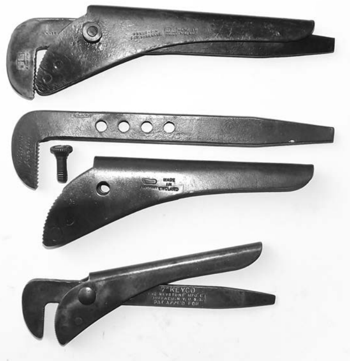
Figure 20a (top and middle) and 20b (bottom). At top is a 7-inch Footprint brand no. 698 plumbers wrench and in the middle is the same wrench in dismantled form. Lower jaw has a hardened steel infill. At bottom is a 7-inch Keyco example of the wrench; the date is unknown.
