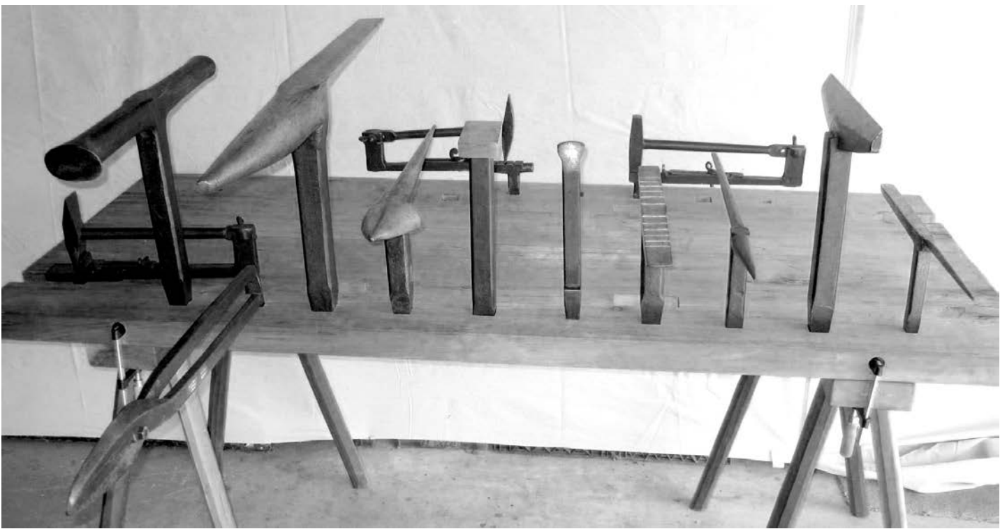
Figure 9 (above). A set of American tinsmith stakes and swedges. From left are a double-seaming stake, square-pen swedge (behind the stake), bench shears, beakhorn stake, blowhorn stake, square stake, bottoming stake, creasing stake, candlemold stake, hatchet stake, and a needlecase stake. At the back of the bench on the left is a creasing swedge and on the right a cullender swedge.
