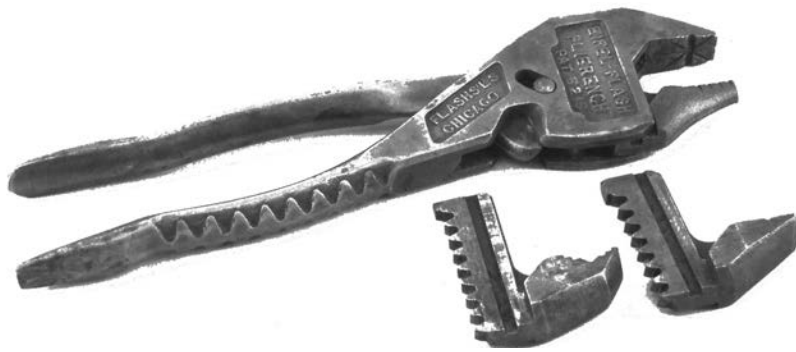
Figure 72 (above). The 8-inch Eifel Flash PlierRench (1920s). Embossed with company name, "Pat.5.2.16," and "FLASH SLS CHICAGO."
