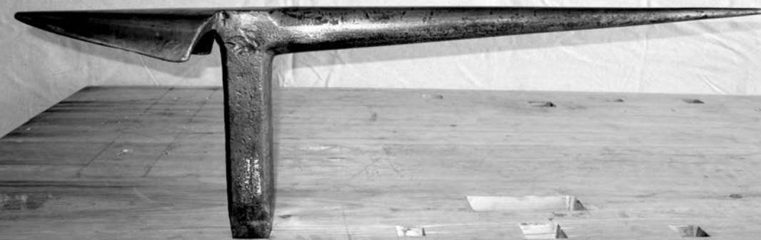
Figure 17 (above). A beakhorn stake marked "J. & E. NORTH /BERLIN CT" circa 1835-1854, 40 inches long.
