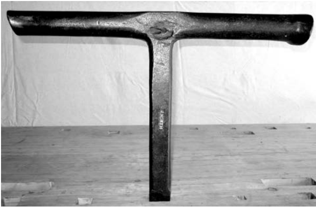
Figure 21 (above). A double-seaming stake marked "J. NORTH" (Berlin, Connecticut), 1810-1824; 21 inches long.
