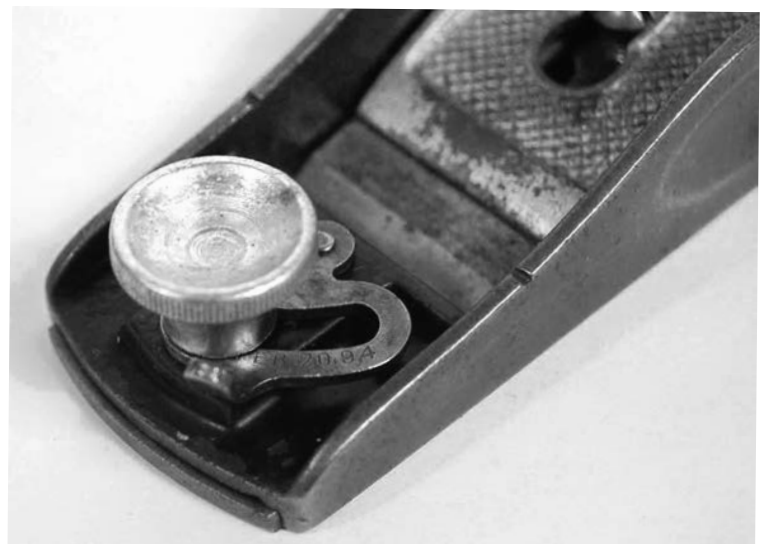
Figure 1 (left). Bodmer’s first patent. Figure 2 (above). Stanley’s no. 60 block plane using Bodmer and Traut’s 1894 patent.
