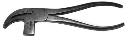
Figure 7 (above, left). A centuries-old, 90-degree, duck bill tong used for handling hot metal fixtures. DRAWING BY KEITH TOWE
