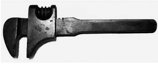
Figure 1 (above). Budding's adjustable spanner, British-registered design no. 7312; May 19, 1843.
