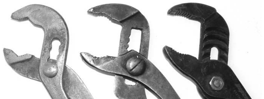
Figure 4. The three most commonly found mechanisms of water pump pliers: slip joint, rack-and-dog joint, and groove-joint.
