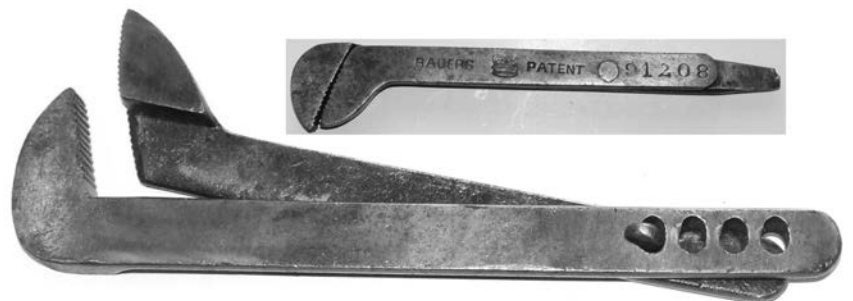
Figure 19. Bauer's patented, 10-inch wrench showing sockets and hooked stud and a 6-inch model (at top). These examples were made in Belgium and are stamped with a crown and patent or design numbers.
