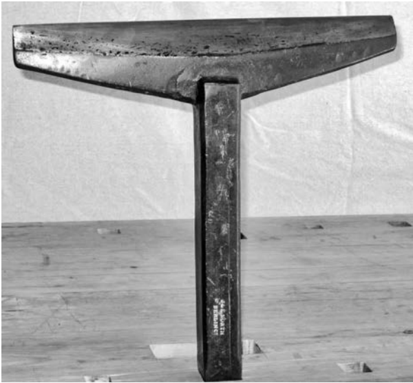
Figure 13 (above). Hatchet stake marked "J. & E. NORTH /BERLIN CT" circa 1835-1854, 14½ inches wide.
