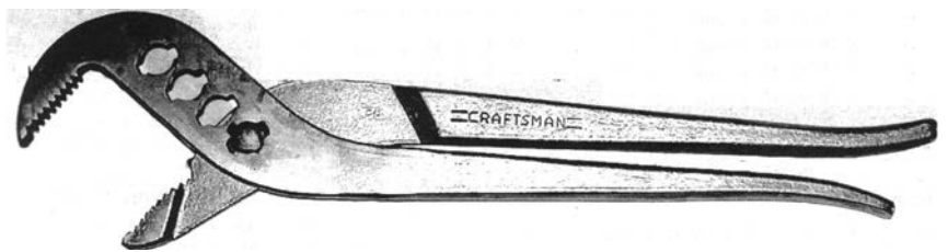
Figure 63 (above). Sears, Roebuck Craftsman brand water pump pliers using T stud connections. MVWC
