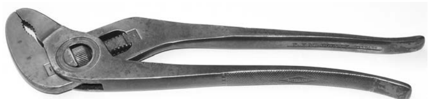
Figure 64 (below). 10¼ inch pliers embossed "CHROM-VANADIUM," "ROT FUB," the patent number, and "GERMANY" on the handles. It is stamped "AMAZONA" below the bolt of the captive leg.
