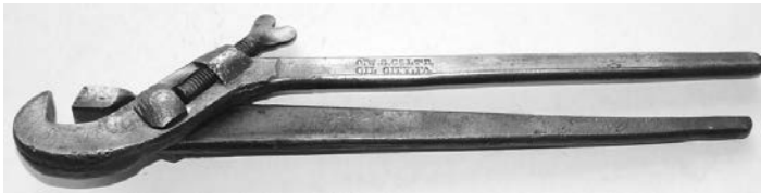
Figure 11 (above). A 15-inch tong, Oil Well Supplies Company, Limited, of Oil City, Pennsylvania, circa 1900. This is virtually identical to Brown's original 1858 patent.
