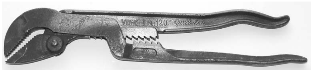
Figure 70 (below) The 12¼-inch VBW Nr. 120 “Griff-Eck” (corner grasp) wrench. It has a 1-inch Whitworth capacity with parallel jaws. The middle leg floats and the racks lock when jaws engage with the nut. It is marked “Crom Vanadium” and “DGDM.”
