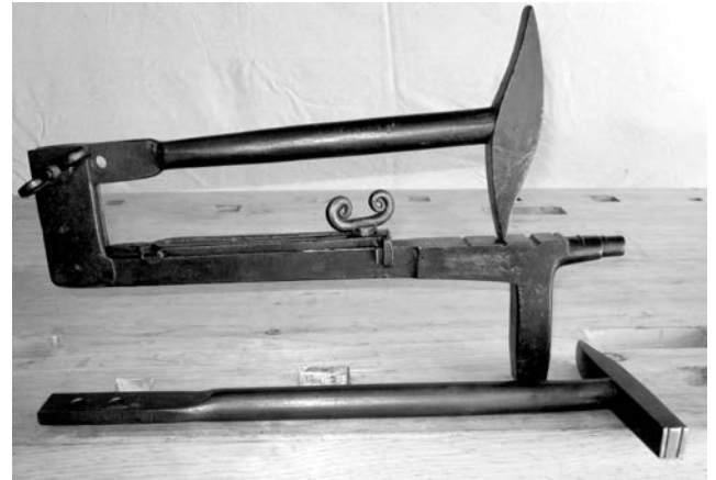
Figure 22 (right, top). A square-pen swedge marked "J.&E. NORTH BERLIN CT" circa 1835-1854.
