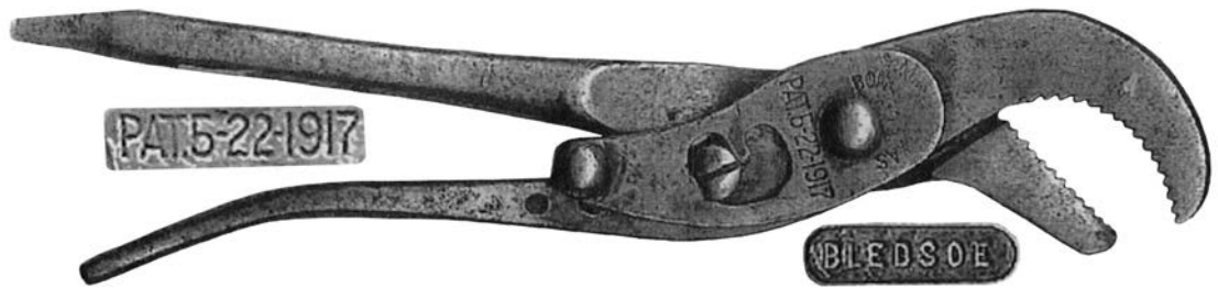
Figure 35 (right). An example of 8-inch Bledsoe pliers with two-position adjusting plate. This patented version does not show manufacturer's location.
