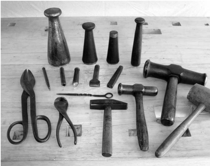
Figure 10 (below). More tools: (top row) hollow punches; (middle row) seam set; rivet set; (bottom row) shears, wire nips, scribe, setting hammer, two raising hammers, and a wooden mallet.
