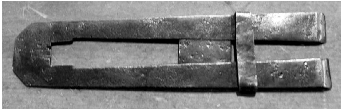
Figures 3 (above) and 4 (below). The iron. The tines are tapered and the metal wedge could be moved up and down in order to change the distance between the cutters.
