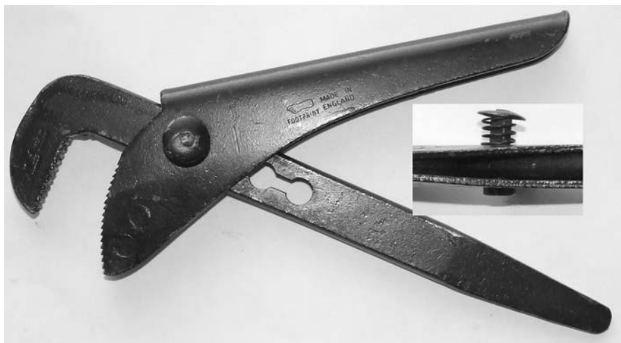
Figure 27a (above). T.R. Ellin's adjustable 9-inch, slip-joint Footprint wrench with locking pin (inset).
