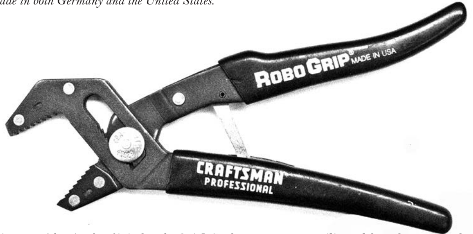
Figure 69 (above). The 6½-inch Robo Grip® Craftsman no. 45028 utility tool from the 1990s and sold through Sears, Roebuck.
