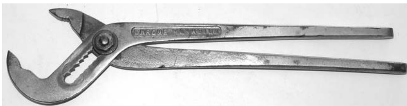
Figure 48 (above, left). J.H. Howard's patented modified footprint. Only marks found are stamped patent number and date, i.e. "21176/24."
