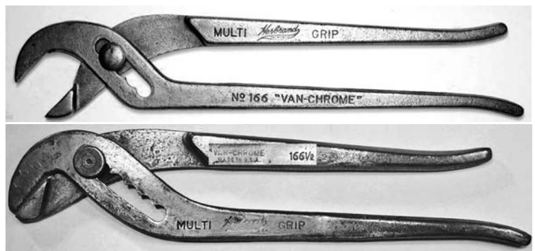
Figure 37. Two pairs of circa 9 1/2-inch Herbrand "MULTIGRIP" pliers. The sockets in the no. 166 model (top) were milled out of the slot front. The no. 166 1/2 model's sockets were milled out of the slot rear.
