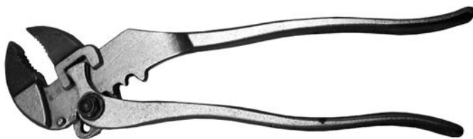
Figure 55. An 8-inch Boker "semi-boxed" lever rack-and-dog pliers. The date is unknown, but it is possibly 1980s.
