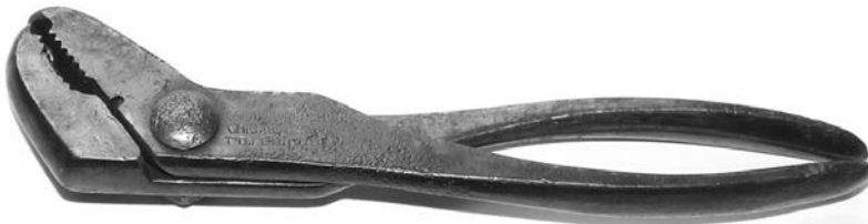
Figure 30 (below). Schlehr's 7½-inch, 45-degree pliers incised "EAGLE CLAW WRENCH CO. CHICAGO. U.S.A. PAT'D FEB 6. 1912" (note date).
